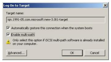
For MPIO connection, you must select the Target that displays status as Connected and select Log On. In the Log On to Target window, select Advanced and configure redundant iSCSI Target IP address.
