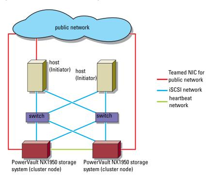
Figure 1-4. Redundant iSCSI Paths Using Four NICs
