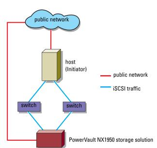
Figure 1-2. Redundant iSCSI Paths With Three NICs
