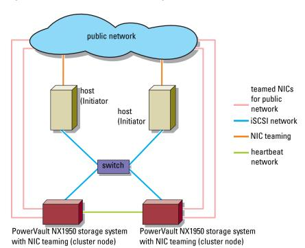
Figure 1-5. Non-Redundant iSCSI Paths Using Four NICs
