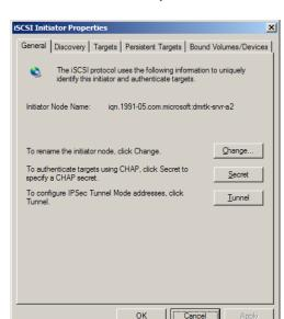
Figure A-1. General Tab in iSCSI Initiator Properties Window
