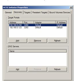
Figure A-2. **Discovery Tab in iSCSI Initiator Properties Window**
